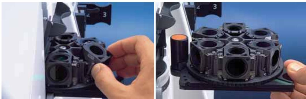
*A matter of seconds: simply exchange reflector modules
