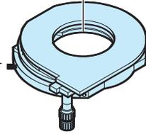
**Rotatable mechanical stage 20x20/90° L**
